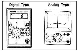
(c) Use a volt/ohmmeter with high impedance (10 k $\Omega$ /V minimum) for troubleshooting of the electrical circuit.
